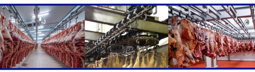
**Overhead Conveyor Chain, Trolleys & Attachments for Red Meat Processing Facilities**
